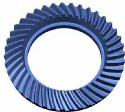
Customized Hypoid Bevel Gear using UG/UFUNC
