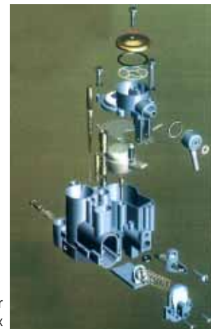
Exploded view of a Carburettor using 3D Studio Max
